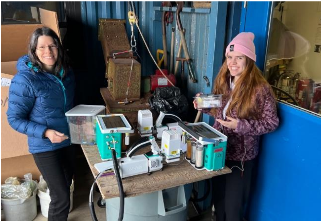
Figure 5- Natasja van Gestel and Sara Bohi Goulart measuring moss photosynthesis with the LI-6800 gas exchange system.
