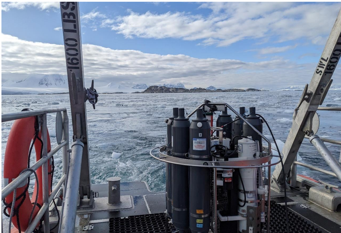
The ECO-Rosette suite of instrumentation for water sampling on board RHIB HADAR at Station E on a calm day, prior to deployment. Image Credit: Hannah James.
